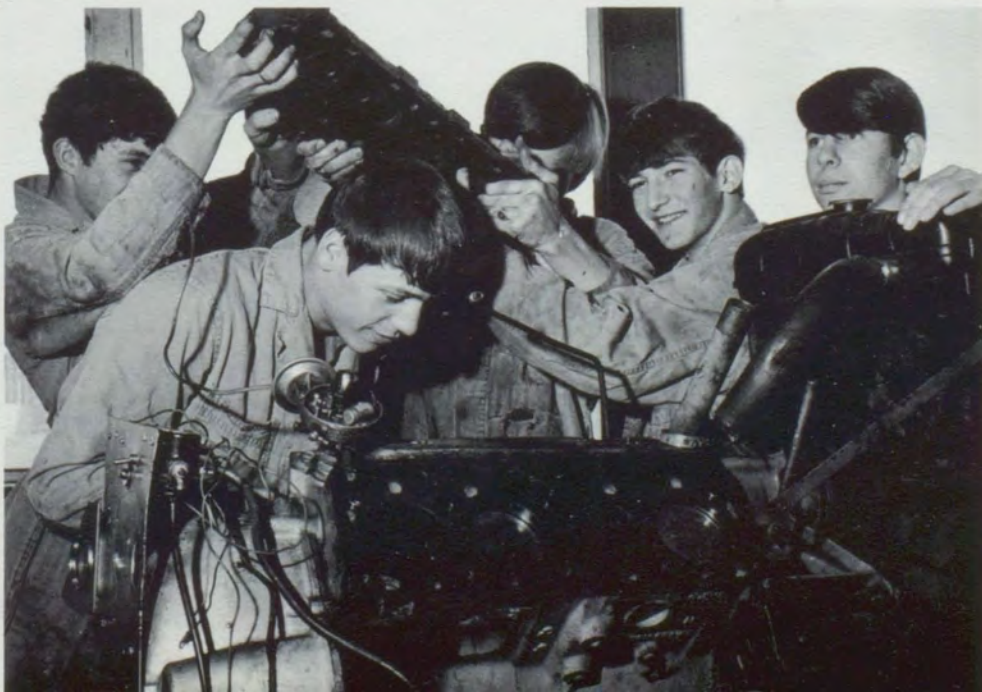
Eugene Townsend, Mike Rice, Dave Kirk, Tim Marr and Mike Busenburg struggle to place the cylinder head on the block. This time removing the forgotten wrench.
