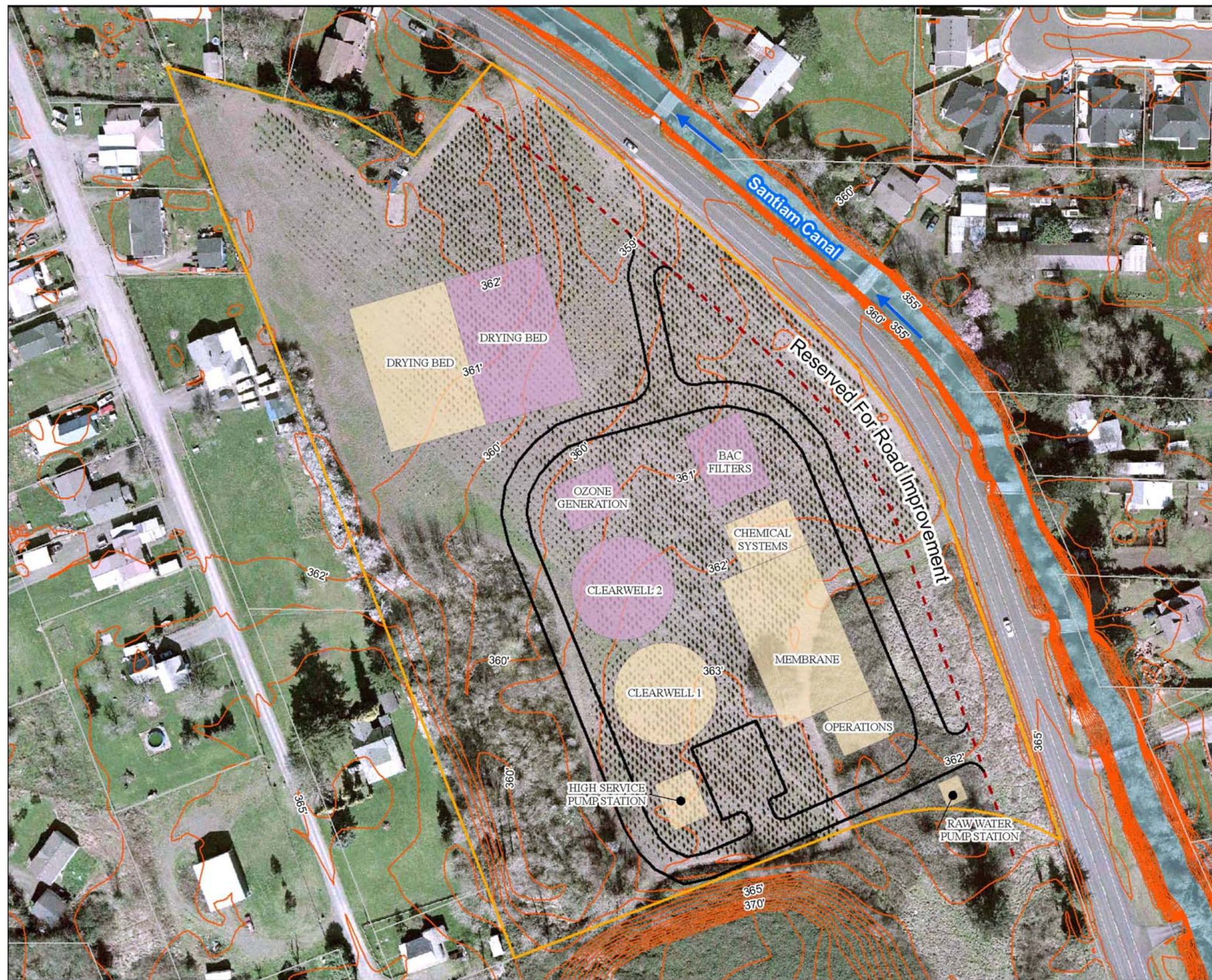
EXHIBIT 5-14 Conceptual Layout for Membrane Filtration Alternative (2 clearwell tanks) City of Lebanon Water Improvement Lebanon, OR
